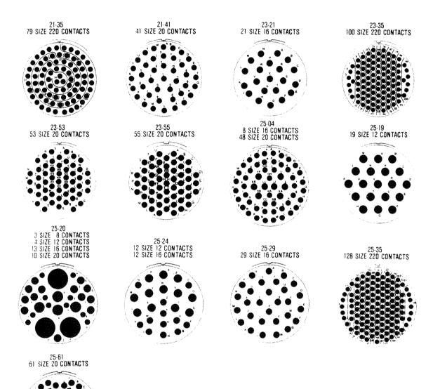
Arrangements are shown looking at pin face (socket is opposite). Cavity identifying letters or numbers are for reference only. Actual marking shall be as required by applicable specifications.
